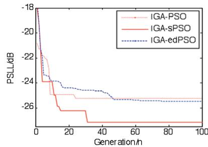
**Figure 6.** Contrast of convergence velocity.
