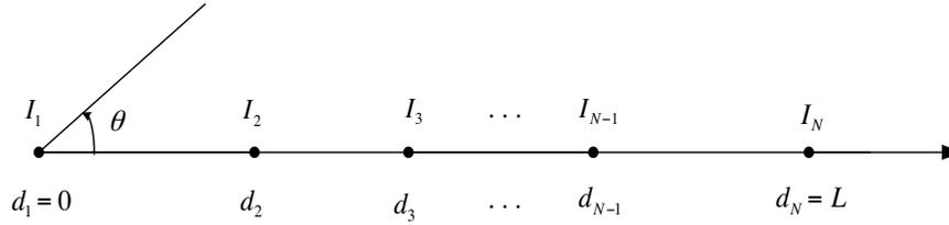
**Figure 1.** Geometry of sparse linear array.
