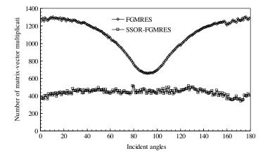
Figure 13. Number of matrix-vector multiplications with FGMRES and SSOR-FGMRES algorithms for the different incident angles (or systems) on the missile.
