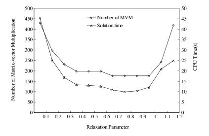
Figure 10. Number of matrix-vector multiplications and solution time with SSOR-FGMRES algorithm for the different relaxation parameters on the open cone example.
