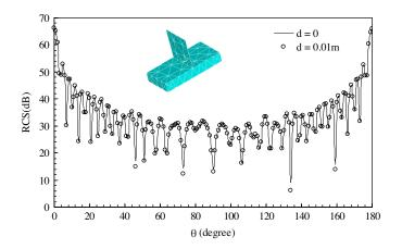
Figure 4. The bistatic RCS at 5 GHz for a box-plate example.
