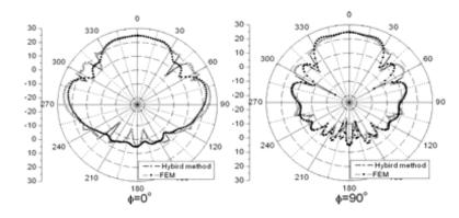
Figure 8. Radiation patterns of the dipole in Fig. 1.
