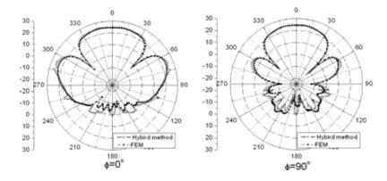
Figure 7. Radiation patterns of the dipole in Fig. 5.
