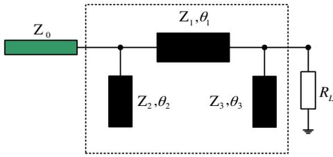
**Figure 1.** Circuit of Pi-structure dual band transformer.
