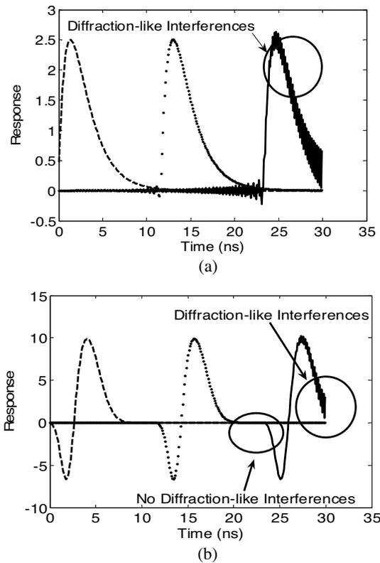
**Figure 3.** Transient waveform of a plane wave propagation at distances of  $\ell = 0, 3.5$  m and  $7$  m. ( $[W_{nm}]_{2 \times 2}$  uses (17)). (a) Equation (27), (b) Equation (28).
