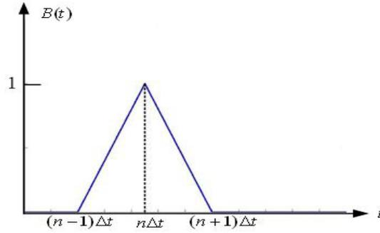
**Figure 2.** A triangular pulse functions.
