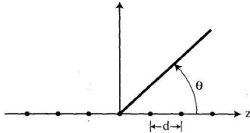
**Figure 2.** Linear array geometry of uniformly spaced isotropic sources.
