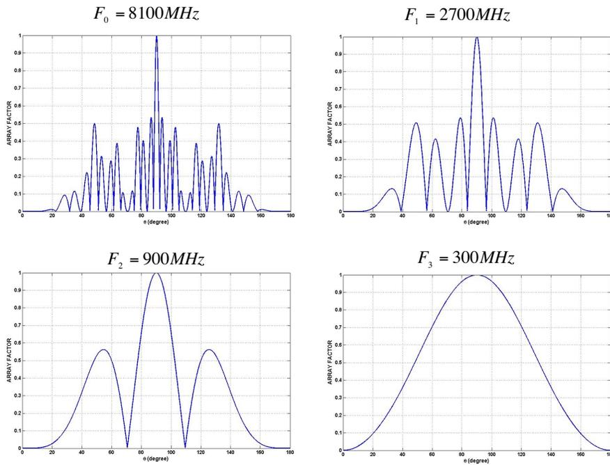
**Figure 4.** Array factor of a fractal Cantor linear array antenna.
