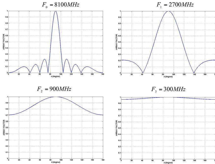
**Figure 5.** Array factor of a conventional non-fractal linear array antenna.
