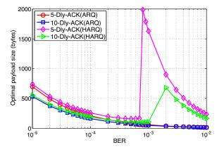
Figure 5. Optimal payload size versus BER for ARQ and HARQ schemes.
