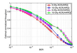
**Figure 4.** Optimal throughput versus BER for ARQ and HARQ schemes.
