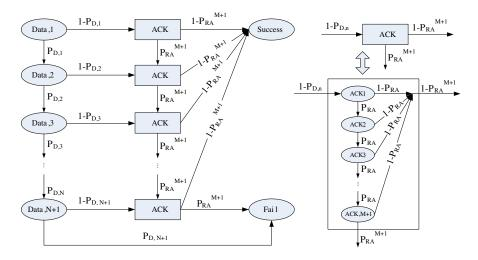
Figure 2. Data transmission process for Dly-ACK mechanism.
