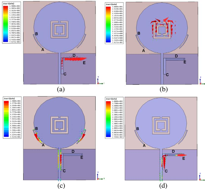
**Figure 6.** HFSS simulated current distributions at: (a) 2.42 GHz, (b) 3.5 GHz, (c) 5.5 GHz, (d) 7.6 GHz.
