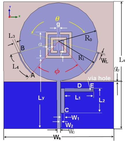
**Figure 1.** Schematic diagram of the proposed antenna.
