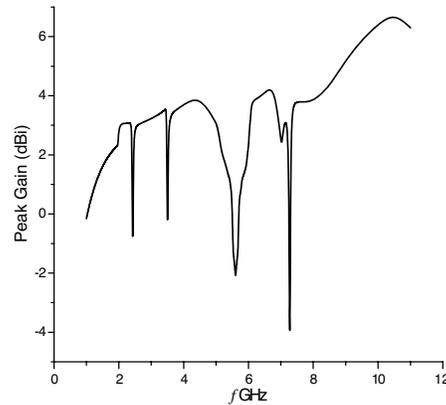
**Figure 7.** The peak gain of the proposed antenna.
