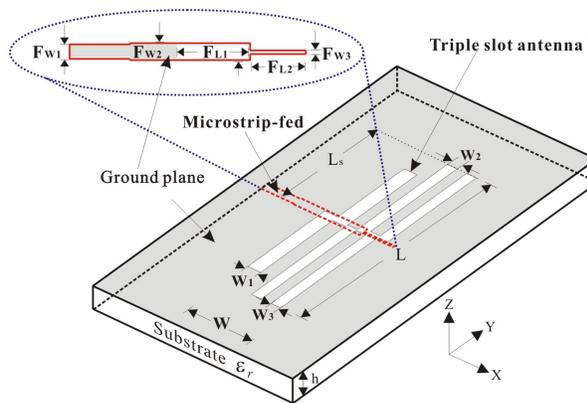
(b) Triple-Z-slot antenna
