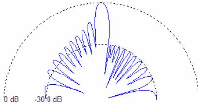
**Figure 2.** Elevation radiation pattern of the antenna.
