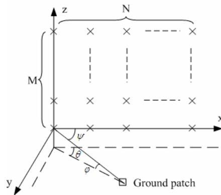
**Figure 1.** Planar array geometry for airborne radar.
