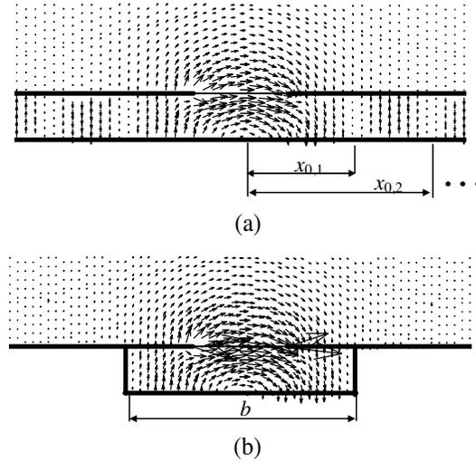
**Figure 2.** Calculated electric field distribution of the dominant mode on the conductor-backed slotline (a), and of the bound mode on the flat slotted waveguide  $b = 2x_0$  in width (b). The normalized frequency is  $h/\lambda_0 = 0.25$ . The line parameters are  $w = 12$  mm,  $h = 6$  mm,  $\varepsilon_r = 2.6$ , the zero field point position is  $x_0 = 14,757$  mm, so  $b = 29.514$  mm.
