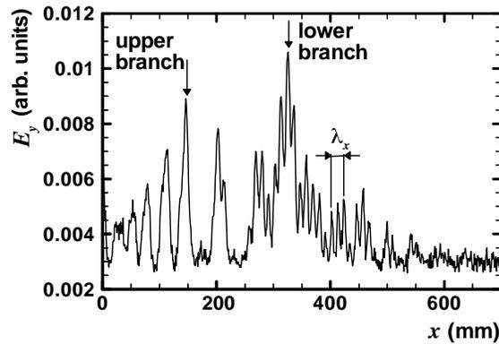
**Figure 9.** Distribution of the electric field measured along the edge of the substrate at the normalized frequency  $h/\lambda_0 = 0.24$ , i.e., 12 GHz for the used substrate. The line with  $w = 12$  mm,  $h = 6$  mm,  $\epsilon_r = 2.6$ .
