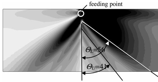
**Figure 8.** The  $E_y$  field distribution calculated by the CST Microwave Studio at the central level  $y = 3$  mm of the substrate of the conductor-backed slotline with  $w = 12$  mm at the normalized frequency 0.18. The conductor-backed slotline is fed through the coaxial line from the left, as shown in Fig. 7.
