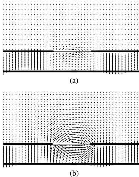
**Figure 11.** The imaginary part of the electric field distribution in the transversal plane of the conductor-backed slotline with a slot 12 mm in width calculated by the APTL code at  $h/\lambda_0 = 0.18$  for the surface leaky mode with higher phase constant  $\beta/k_0 = 1.252$  (a), and with lower phase constant  $\beta/k_0 = 0.923$  (b).
