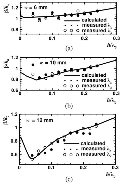
**Figure 3.** Calculated and measured normalized dispersion characteristics of the dominant mode on the lines with  $h = 6$  mm, permittivity 2.6 and different  $w$ . The way of obtaining the experimental results is described in paragraph 4.1.
