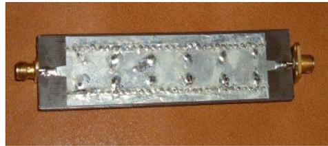
**Figure 4.** Photograph of the manufactured five-pole Chebyshev filter.
