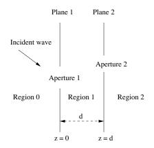
Figure 2. Setup and notations for problem of transmission through apertures through a two-parallel-plate region.
