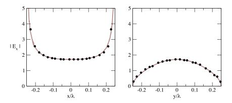
**Figure 4.** Magnitude of  $E_x$  in the  $\lambda/2 \times \lambda/2$  aperture, sampled along the  $(O, \vec{u}_x)$  and  $(O, \vec{u}_y)$  axis. Dots represent results from the present method and the thick line those calculated with FDTD software.
