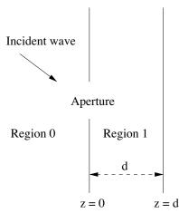
Figure 1. Setup and notations for problem of coupling through an aperture in a two-parallel-plate region.
