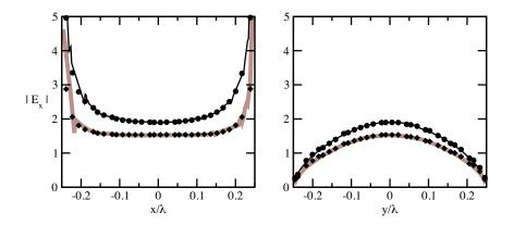
**Figure 5.** Magnitude of  $E_x$  in the  $\lambda/2 \times \lambda/2$  apertures, sampled along the axis. Continuous lines represent the output of FDTD software in the left (thin black) and right (thick grey) apertures, the squares and diamonds represent the output of the present method in the left and right apertures respectively.
