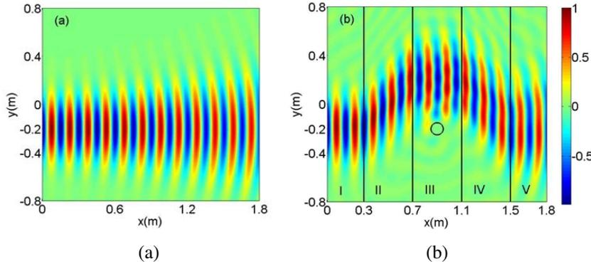
**Figure 2.** Normalized electric field distribution in (a) free space as reference (b) a set of beam shifters with  $b = 1$ . Regions I, III, V are free space; region II is an up-shifter; region IV is a down-shifter. The Gaussian beam was centered at  $y = -0.2$  m.
