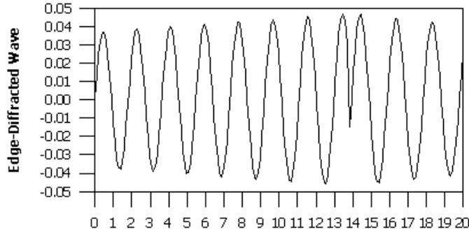
**Figure 4.** Variation of the edge diffracted wave with normalized time.
