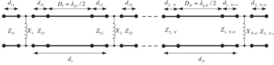
**Figure 4.** Transmission line realization of a dielectric filled waveguide bandpass filter.
