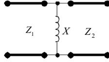
**Figure 6.** The equivalent circuit of a diaphragm.
