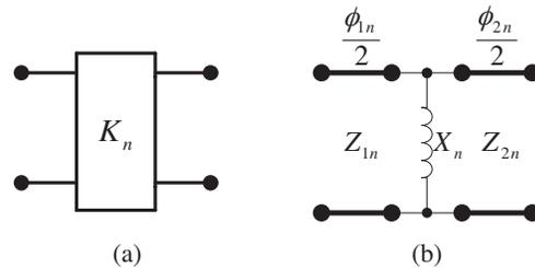
**Figure 3.** (a) An impedance inverter. (b) A circuit model for impedance invertors.
