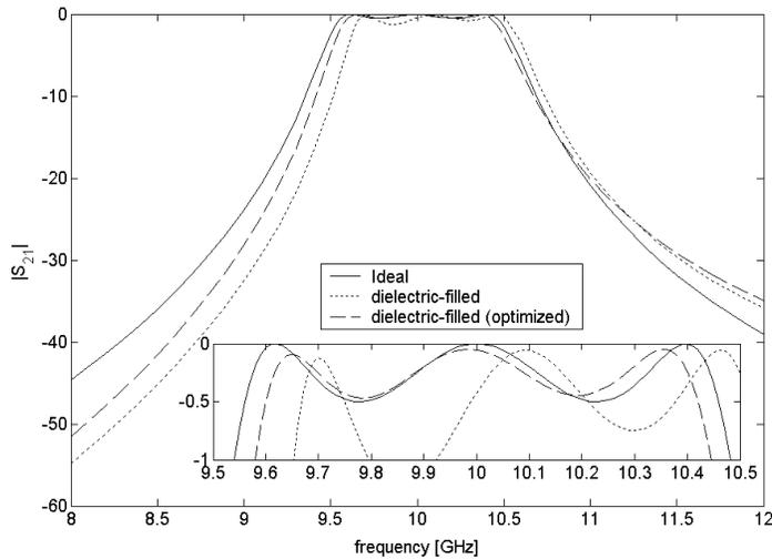
**Figure 8.** The simulation results of designed dielectric-filled waveguide bandpass filter.
