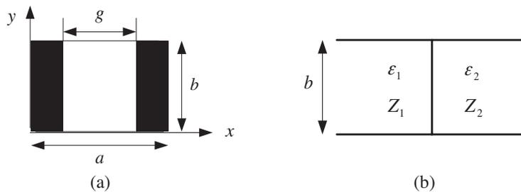
**Figure 5.** (a) The cross sectional view of a diaphragm. (b) The side view of a diaphragm.
