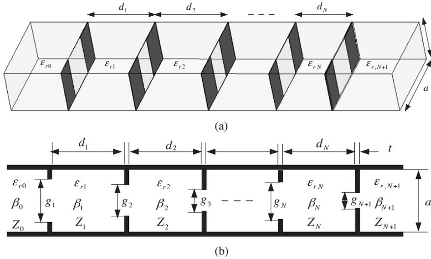
**Figure 1.** The proposed dielectric filled waveguide bandpass filter. (a) Three dimensional view. (b) Top view.
