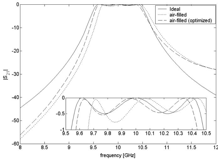
**Figure 7.** The simulation results of designed air-filled waveguide bandpass filter.
