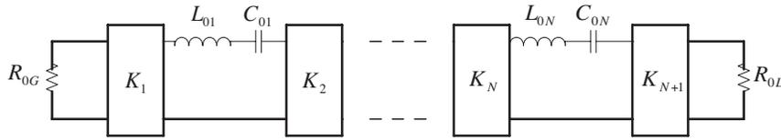
**Figure 2.** Typical bandpass filter using series resonators and impedance invertors.
