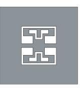
Figure 10. Ground plane of the dual-band bandpass filter.
