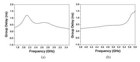
Figure 14. Group delay in the two passbands: (a) the lower passband, (b) the upper passband.
