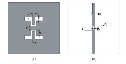
**Figure 4.** Layout of back-to-back filter: (a) view of the ground plane, (b) view of the signal plane.
