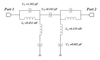
Figure 6. An equivalent circuit model for the back-to-back bandpass filter.
