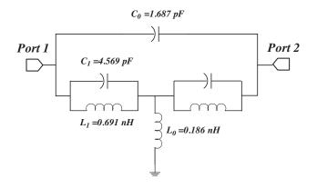
Figure 9. An equivalent circuit model for the face-to-face bandpass filter.
