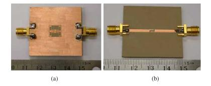
**Figure 12.** Photograph of the fabricated filter: (a) view of the ground plane, (b) view of the signal plane.
