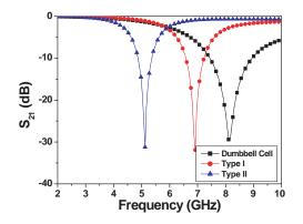
Figure 2. Simulated  $S_{21}$  of the three structures (as drawn in Fig. 1) with the same rectangular occupying area.
