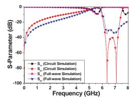
**Figure 5.** Simulated results of the back-to-back bandpass filter by *IE3D* and *ADS*.
