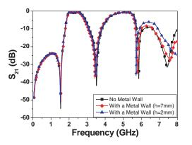
Figure 15. The effect of a closely placed metal wall on the dual-band bandpass filter using slotted ground structures.
