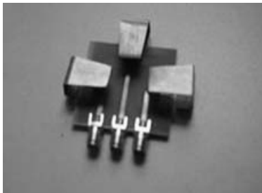
Figure 3. Photograph of the planar inverted-L diversity antenna.
