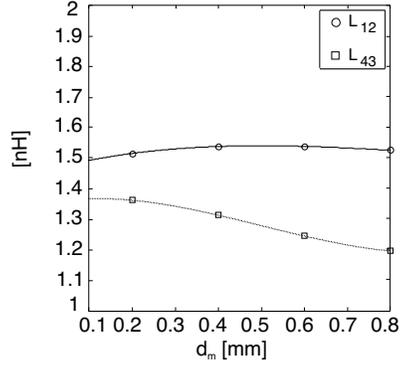
**Figure 6.** Values of the inductors of the proposed equivalent circuit (*symbols*) and their interpolant polynomial functions (*lines*) versus  $d_m$ .
