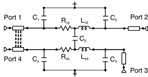
**Figure 2.** Equivalent circuit of the straight-to-bent microstrip line coupling problem.
