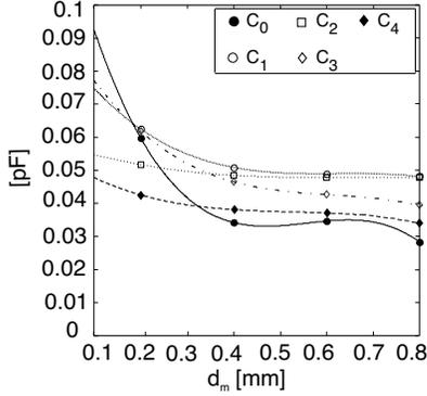
**Figure 5.** Values of the capacitors of the proposed equivalent circuit (*symbols*) and their interpolant polynomial functions (*lines*) versus  $d_m$ .
