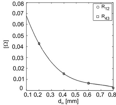
**Figure 7.** Values of the resistors of the proposed equivalent circuit (*symbols*) and their interpolant polynomial functions (*lines*) versus  $d_m$ . The resistors  $R_{12}$  and  $R_{43}$  presents similar values for the structure analyzed.
