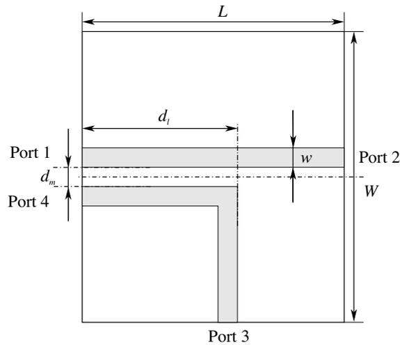
**Figure 1.** Geometry of the straight-to-bent microstrip line coupling problem.
