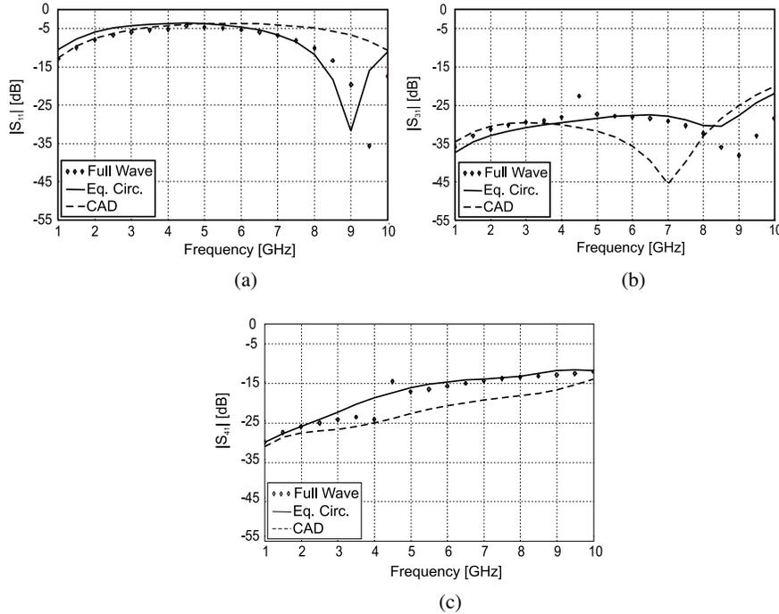
**Figure 3.** Magnitude of the scattering parameters versus frequency for  $d_m = 0.4$  mm,  $d_l = 3.75$  mm. Full wave analysis (*circles*); CAD simulator (*dashed line*); CAD simulator enhanced with the proposed equivalent circuit (*continuous line*): (a)  $S_{11}$ , (b)  $S_{31}$ , and (c)  $S_{41}$ .
