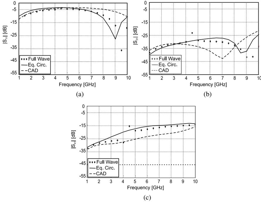
**Figure 4.** Magnitude of the scattering parameters versus frequency for  $d_m = 0.6$  mm,  $d_l = 3.75$  mm. Full wave analysis (*circles*); CAD simulator (*dashed line*); CAD simulator enhanced with the proposed equivalent circuit (*continuous line*): (a)  $S_{11}$ , (b)  $S_{31}$ , and (c)  $S_{41}$ .
