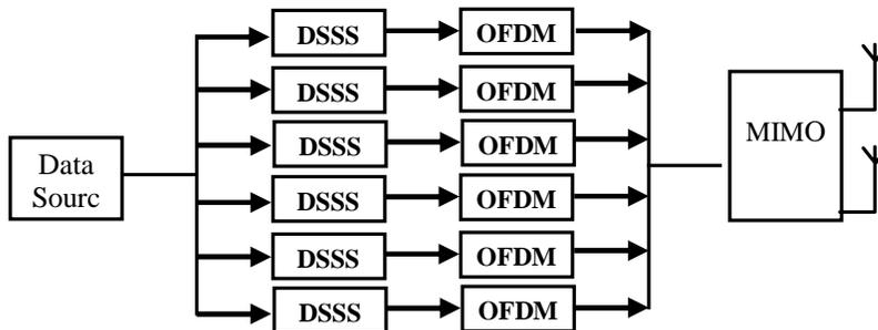
**Figure 2.** Simplified block diagram of COFDM-MIMO system.
