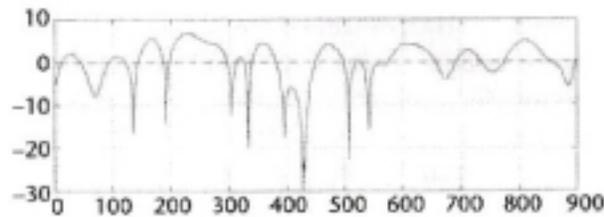
**Figure 1.** Signal fading due to multipath effect.
