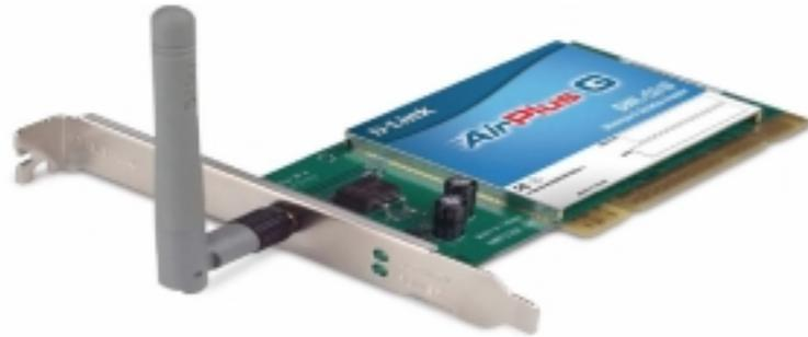
**Figure 3a.** Photograph of PCI Wi-Fi b/g adapter.
