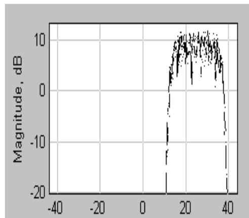
**Figure 3b.** The received signal spectrum from a DSSS system.
