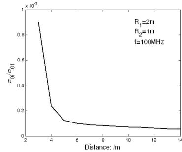
**Figure 8.** Complex RCS versus the distance.
