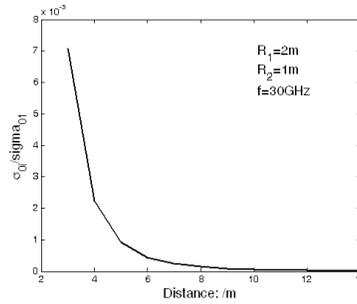
**Figure 9.** Complex RCS versus the distance.
