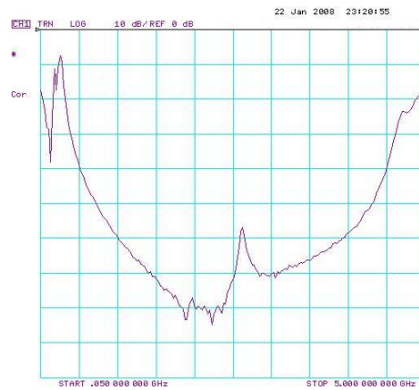
Figure 5. Measured |S_{31}| of EBG structure.
