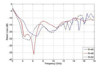
Figure 6. Simulated return loss of the antenna for various R.  $2a = 19.5 \text{ mm}, 2b = 31.4 \text{ mm}, l = 7.1 \text{ mm}, W = 2 \text{ mm}, h = 2.3 \text{ mm}, r = 2.6 \text{ mm} \text{ and } \alpha = 45^{\circ}.$
