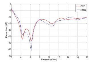
Figure 2. Simulated return loss of the proposed antenna. 2a = 19.5 mm, 2b = 31.4 mm, l = 7.1 mm, W = 2 mm, R = 46 mm, h = 2.3 mm, r = 2.6 mm and  $\alpha = 45^{\circ}$ .
