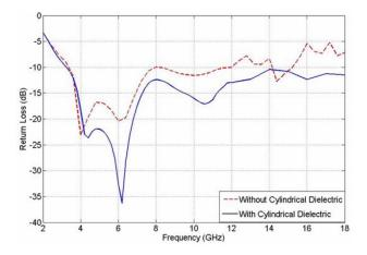
Figure 7. Simulated return loss of the proposed antenna with and without dielectric.  $2a = 19.5 \text{ mm}, 2b = 31.4 \text{ mm}, l = 7.1 \text{ mm}, W = 2 \text{ mm}, R = 46 \text{ mm}, h = 2.3 \text{ mm}, r = 2.6 \text{ mm} \text{ and } \alpha = 45^{\circ}.$
