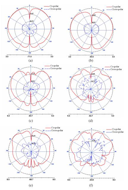
**Figure 3.** Simulated radiation patterns at: 3 GHz in (a) x-z plane, (b) y-z plane, 10 GHz in (c) x-z plane (d) y-z plane, 18 GHz in (e) x-z plane, (f) y-z plane.  $2a = 19.5 \text{ mm}, 2b = 31.4 \text{ mm}, l = 7.1 \text{ mm}, W = 2 \text{ mm}, R = 46 \text{ mm}, h = 2.3 \text{ mm}, r = 2.6 \text{ mm} \text{ and } \alpha = 45^{\circ}.$
