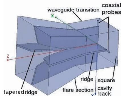
**Figure 1.** Configuration of the quad ridged horn antenna.
