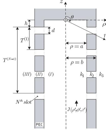
**Figure 1.** Geometry of problem. inner and outer radii:  $a$  and  $b$ , number of slots:  $N$ , width of the slot:  $d$ , distance from the top of  $q$ -th slot to the top of 1st slot:  $T^{(q-1)}$ , wave numbers of regions (I), (II), and (III):  $k_1 = \omega\sqrt{\mu_1\epsilon_1}$ ,  $k_2 = \omega\sqrt{\mu_2\epsilon_2}$  and  $k_3 = \omega\sqrt{\mu_3\epsilon_3}$ .
