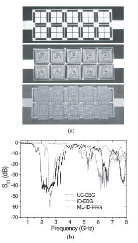
Figure 2. (a) Photograph of top side of there EBG structures connected with microstrip lines and (b) measured  $S_{21}$  parameters of these EBG structures.
