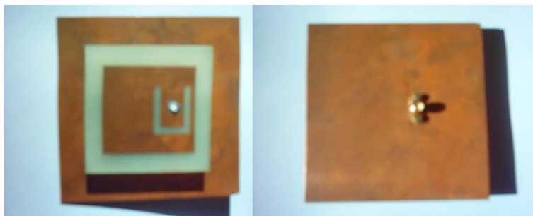
Figure 19. The fabricated antenna front view (left) and back view (right).
