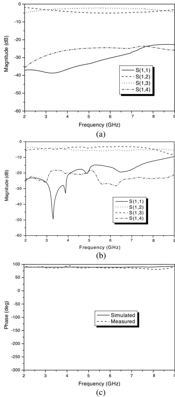
**Figure 8.** Scattering parameters of the proposed coupler (a) simulated, (b) measured, (c) phase difference.
