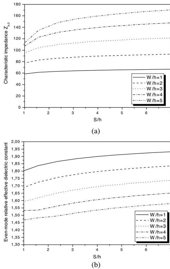
**Figure 4.** (a) Even-mode characteristic impedance, (b) effective permittivity as a function of  $S$  and  $W/h$ .
