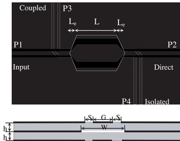
**Figure 7.** Layout of the proposed CPW hexagonal slot coupled directional coupler.
