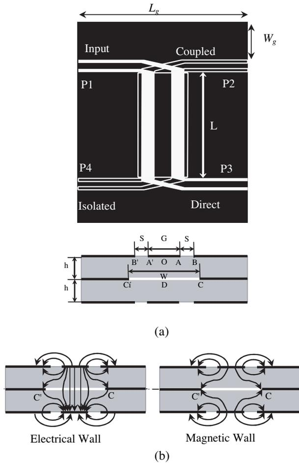
**Figure 1.** Broadside directional slot-coupled coupler: (a) layout, (b) odd and even-mode electric field distribution.
