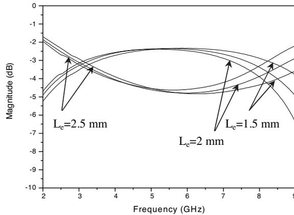
**Figure 9.** Simulated of the scattering parameters of the coupler versus  $L_c$ .
