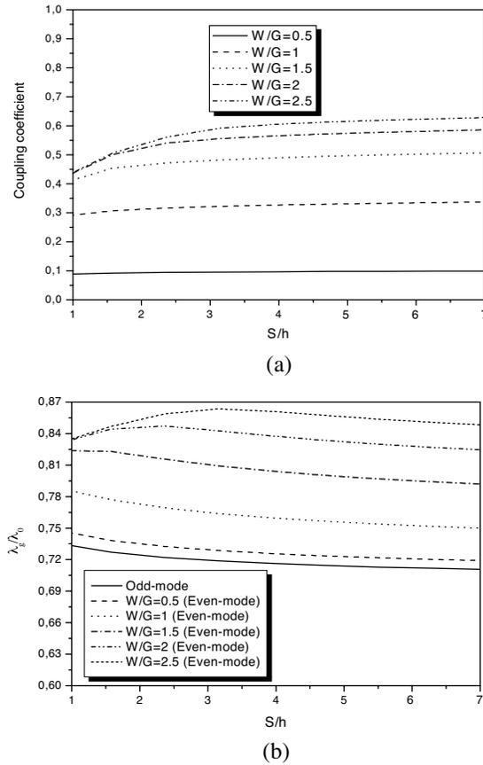
**Figure 6.** (a) Coupling coefficient, (b) normalized wavelength of even and odd modes.
