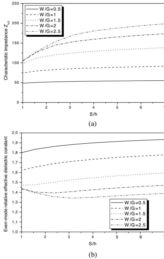
**Figure 5.** (a) Even-mode characteristic impedance, (b) and effective permittivity as a function of  $S$  and  $W/G$ .
