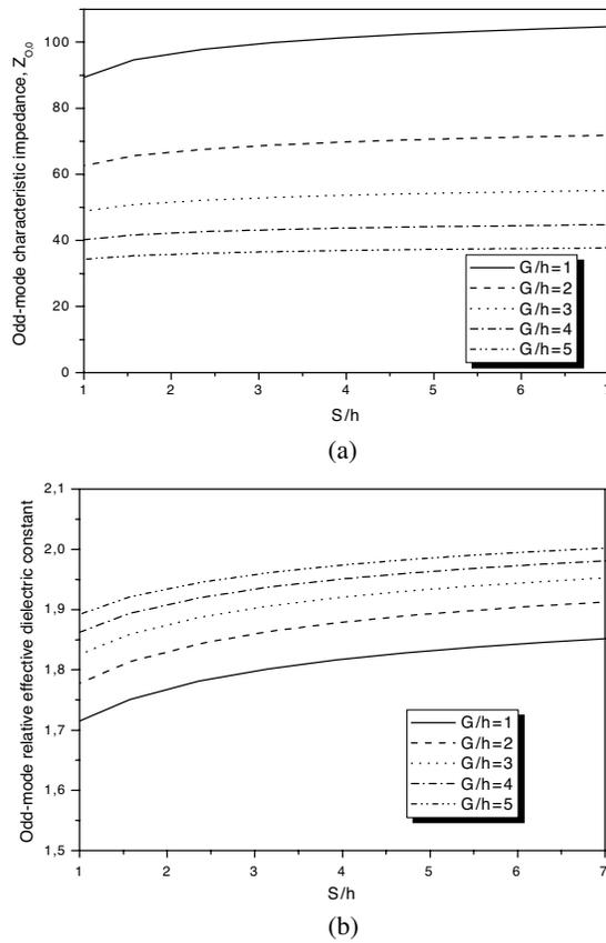
**Figure 3.** (a) Odd-mode characteristic impedance, (b) effective permittivity.
