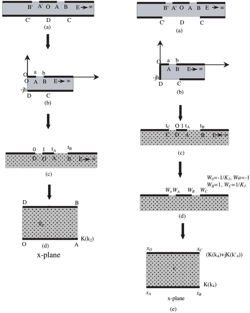
**Figure 2.** Conformal mapping transformation of the odd- and even-mode (dielectric region).
