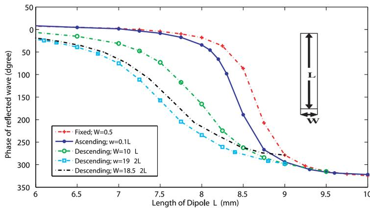
**Figure 5.** Phase response for a dipole of length ( $L$ ) for various schemes of width ( $W$ ) variation.
