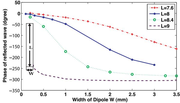
**Figure 4.** Phase response of various fixed-length ( $L$ ) dipoles against the width ( $W$ ).
