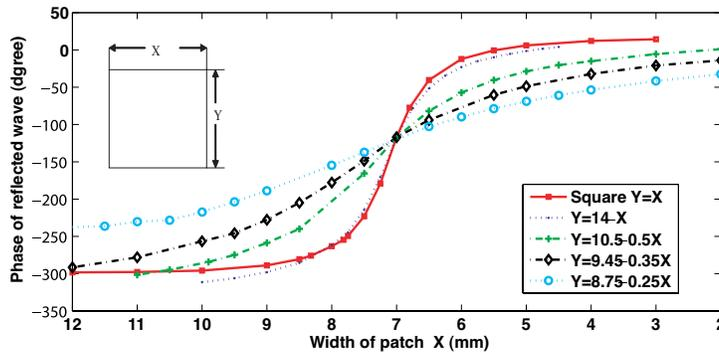
**Figure 6.** Phase response for square patches against dimension perpendicular to the electric field for the various schemes of length variations.
