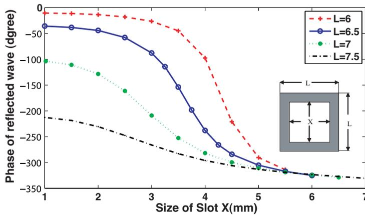
**Figure 1.** Phase response of fixed-size ( $L$ ) square patches against slot size ( $X$ ).
