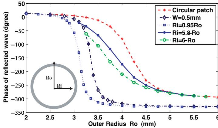
**Figure 8.** Phase response for circular rings against outer radius ( $R_o$ ) for various schemes of varying the slot size.
