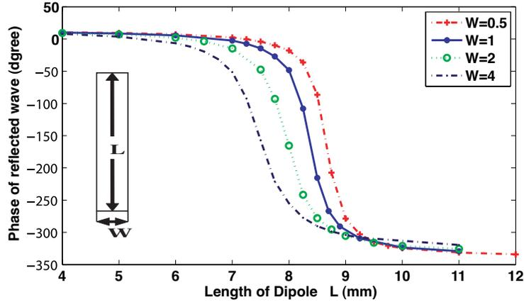
**Figure 3.** Phase response of dipoles for various fixed widths ( $W$ ).
