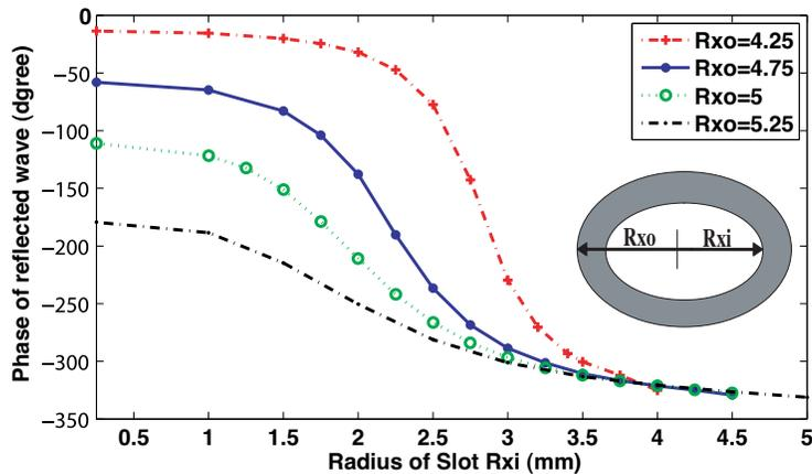
**Figure 2.** Phase response of fixed-size elliptical patches against slot radius  $R_{xi}$ , ( $Dy/Dx = 0.8$ ).
