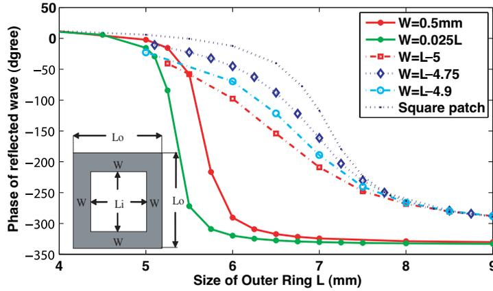
**Figure 7.** Phase response for square rings against outer size ( $L$ ) for various schemes of varying the width  $W$ .
