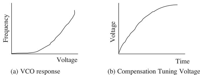
**Figure 2.** Nonlinear frequency response of a VCO (a) and the required compensation tuning voltage (b).
