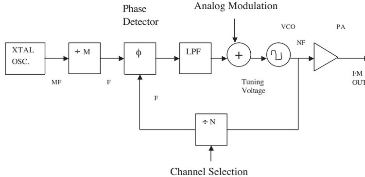
**Figure 1.** A basic block diagram of a traditional analog FM modulation oscillator.
