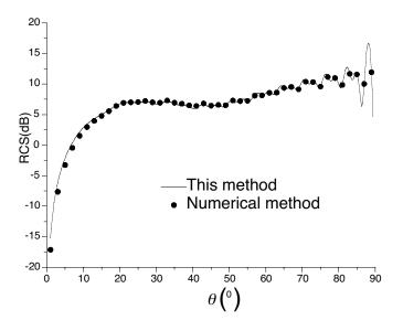
Figure 5. RCS of the cylindrically curved plate.
