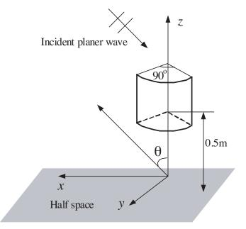
Figure 4. Geometry of a cylindrically curved plate.
