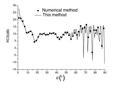
Figure 3. RCS of the spherically curved plate.
