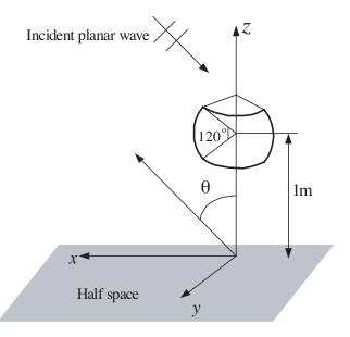
Figure 2. Geometry of a spherically curved plate.
