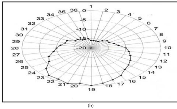
**Figure 8.** Characteristic simulation for  $H = 3\text{ mm}$  (a)  $S_{11}$  (b) Radiation pattern.
