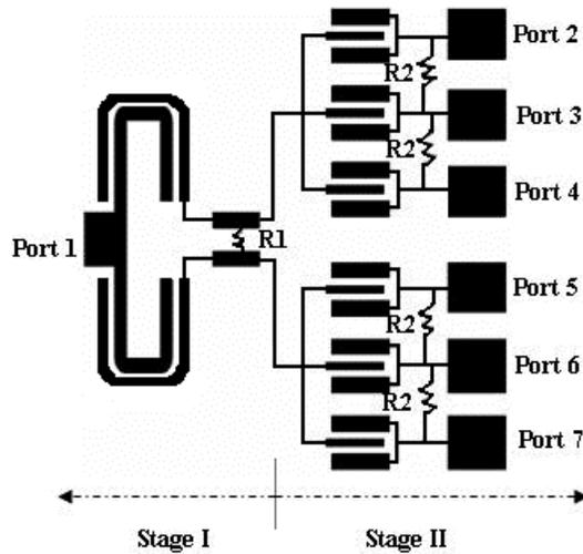
**Figure 1.** The circuit topology of the proposed six-way power divider.
