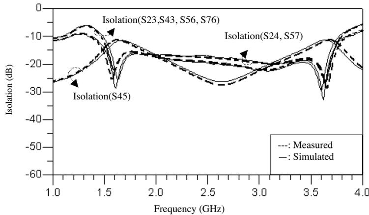
**Figure 8.** Simulated and the measured isolation of the power divider.
