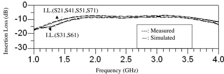
**Figure 6.** Simulated and the measured insertion loss of the power divider.
