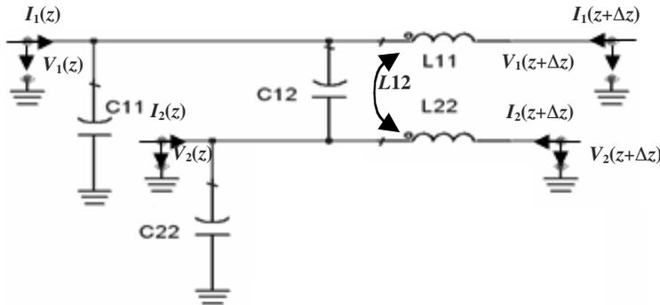
(c) Equivalent circuit topology of the two lossless coupled unit
