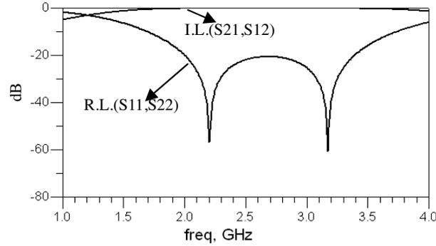
**Figure 4.** Simulated results of two-coupled transmission line behavior.
