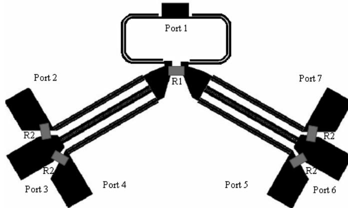
**Figure 5.** The six-way power divider PCB layout.
