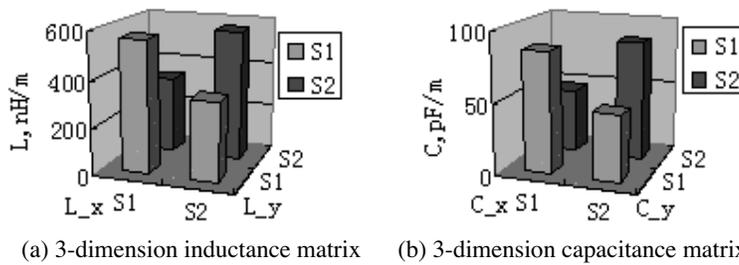
**Figure 3.** Calculated characteristic parameters of two-coupled transmission line.
