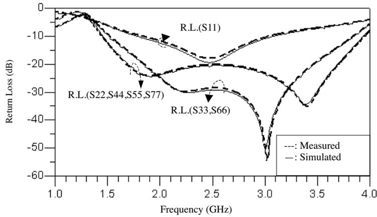
**Figure 7.** Simulated and the measured return loss of the power divider.
