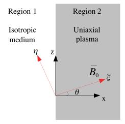
Figure 1. Diagram for an interface between a semi-infinite isotropic medium and a uniaxial plasma. The  $\xi$  axis indicates principle axis, also the direction of the external magnetic field which is infinitely strong in the uniaxial plasma.
