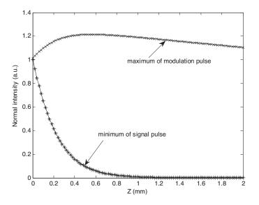
Figure 3. Variety curves of signal pulse minimum and modulation pulse maximum against the length of silicon WG.
