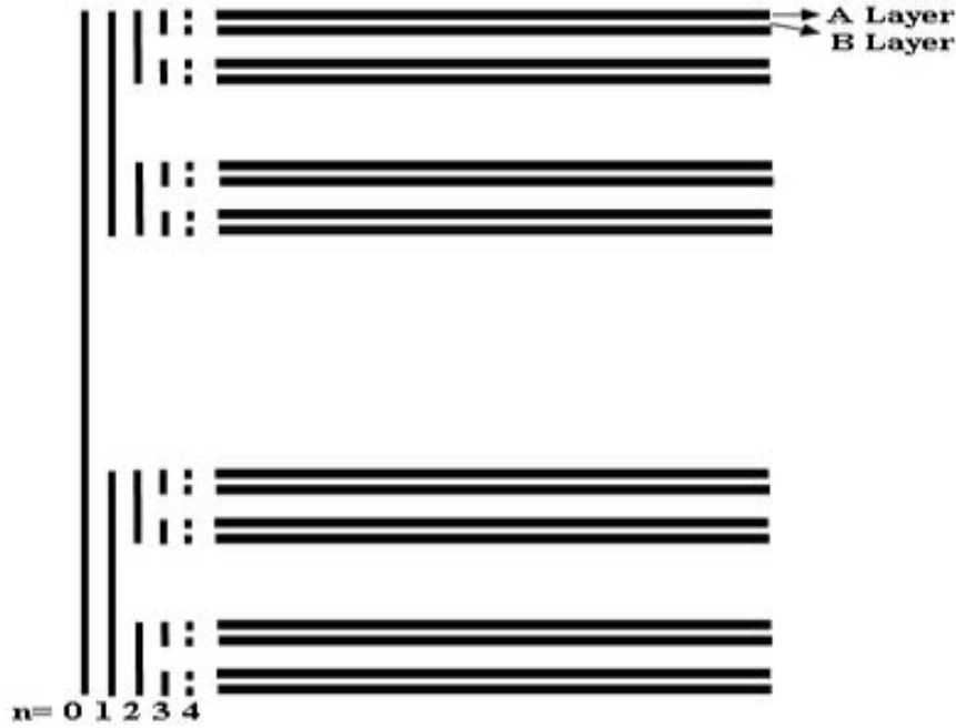
Figure 9. A pseudo periodic dielectric multilayer cantor superlattice with fractal dimension \ln 2 / \ln 3 .
