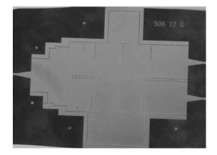
Figure 5. Photograph of the generalized chebyshev SIW diplexer.
