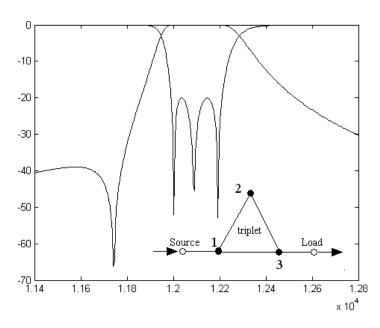
Figure 2. Frequency response of 3th order filter with transmission zeros below the passband.
