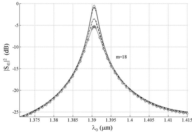
**Figure 7.** Comparison between different loss factors for the computed coupled power at the drop port: for  $\tan(\delta) = 0$  (solid line),  $\tan(\delta) = 0.0001$  (dotted line),  $\tan(\delta) = 0.0006$  (dashed line), and  $\tan(\delta) = 0.001$  (diamond-line).
