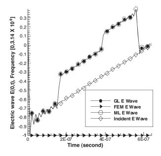
**Figure 5.** GL, ML and FEM electric wave E(0,t) in time domain.
