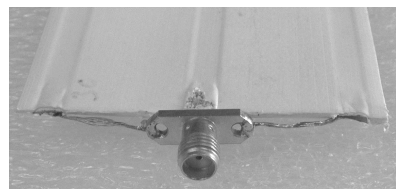
(b) The coaxial connector.
