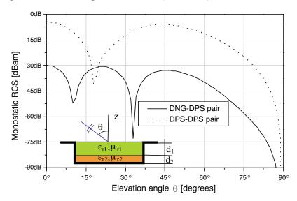
**Figure 2.** Monostatic RCS  $\sigma_{\theta\theta}$  at f=5 GHz for a  $\theta$ -polarized incident plane wave. The cavity dimensions are:  $10 \text{ cm} \times 10 \text{ cm} \times 1.5 \text{ cm}$ ; while the slab parameters are:  $d_1=1 \text{ cm}$ ,  $d_2=0.5 \text{ cm}$ ,  $\varepsilon_{r1}=\pm 2$ ,  $\mu_{r1}=\pm 1$ ,  $\varepsilon_{r2}=4$ ,  $\mu_{r2}=2$ .
