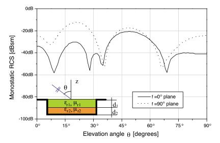
**Figure 5.** Monostatic RCS  $\sigma_{\theta\theta}$  for a  $\varphi$ -polarized incident plane wave at  $f=10\,\mathrm{GHz}$ . The cavity dimensions are:  $10\,\mathrm{cm}\times 10\,\mathrm{cm}\times 1.5\,\mathrm{cm}$ ; while the slab parameters are:  $d_1=1.02\,\mathrm{cm},\ d_2=1.02\,\mathrm{cm},$   $\varepsilon_{r1}=9.957,\ \mu_{r1}=0.037,\ \varepsilon_{r2}=5.747,\ \mu_{r2xx}=\pm 0.283,\ \mu_{r2yy}=-0.283,\ \mu_{r2zz}=0.283.$
