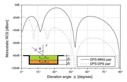
**Figure 3.** Monostatic RCS  $\sigma_{\theta\theta}$  at  $f=10\,\mathrm{GHz}$  for a  $\theta$ -polarized incident plane wave. The cavity dimensions are:  $10\,\mathrm{cm}\times10\,\mathrm{cm}\times1.5\,\mathrm{cm}$ ; while the slab parameters are:  $d_1=1.02\,\mathrm{cm},\ d_2=1.02\,\mathrm{cm},\ \varepsilon_{r1}=9.957,\ \mu_{r1}=0.037,\ \varepsilon_{r2}=5.747,\ \mu_{r2}=\pm0.283.$
