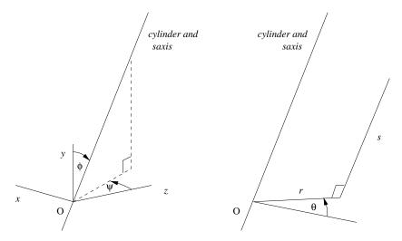
**Figure 2.** Target orientation and coordinate system: O' is an origin on the cylinder axis and the Cartesian x'y'z'-axes are parallel to the original xyz-axes of Figure 1. When the x'y'z'-axes are rotated through  $\phi$  about  $u = \cos \psi e^{(1)} - \sin \psi e^{(3)}$ , which is normal to the vertical plane containing the cylinder's axis, the y'-axis is rotated to the *s*-axis and the y'z'-coordinate plane is rotated to the  $\theta = 0$  plane of the cylindrical coordinate system.
