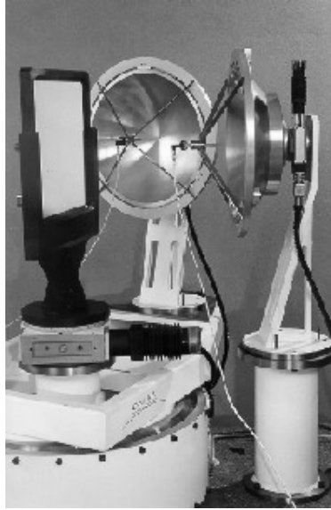
Figure 22. Measurements setup in Ka-band.
