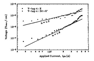
Figure 8. Measured in-phase and quadrature voltages using contact (4) against peak applied current.
