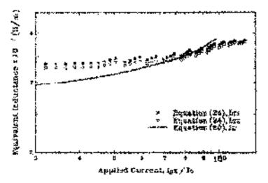
Figure 3. Measured and calculated equivalent inductance variation with applied current in the 7-filament tape at 256 Hz. second set of data  $(L_{T2})$  demonstrates the reproducibility of the measurements to within 2%.
