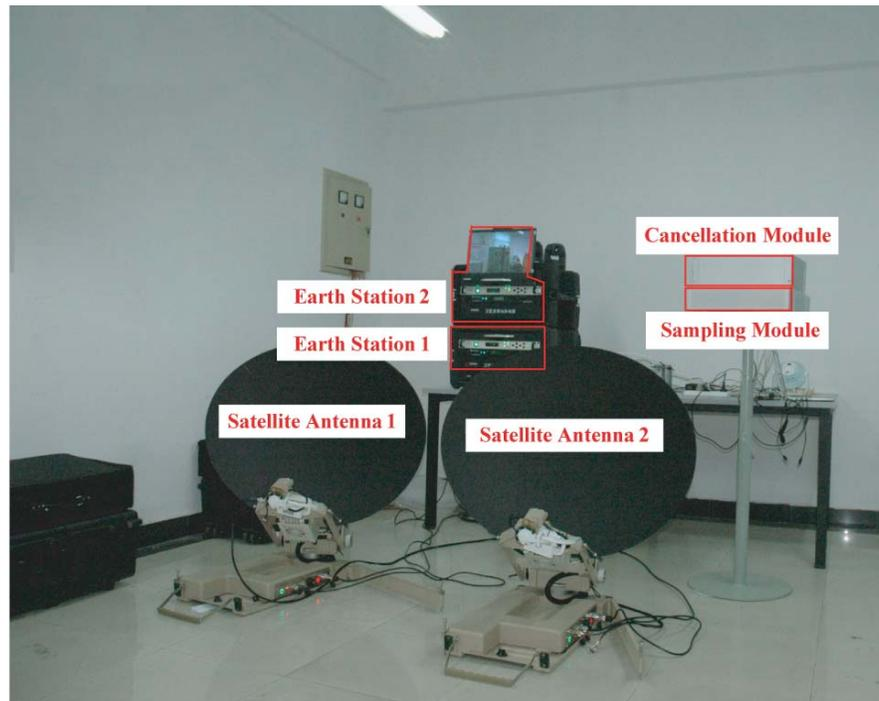
**Figure 10.** Satellite interference cancellation experiment system.
