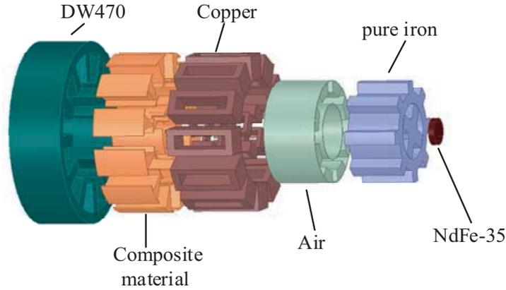
**Figure 5.** 3D thermal model.
