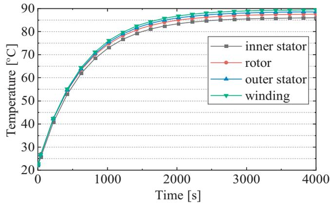
**Figure 8.** Temperature rise curve.
