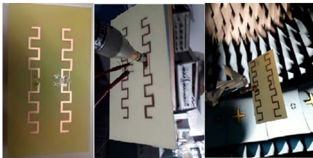
Figure 14. Photograph of the prototype of super directive reconfigurable antenna.
