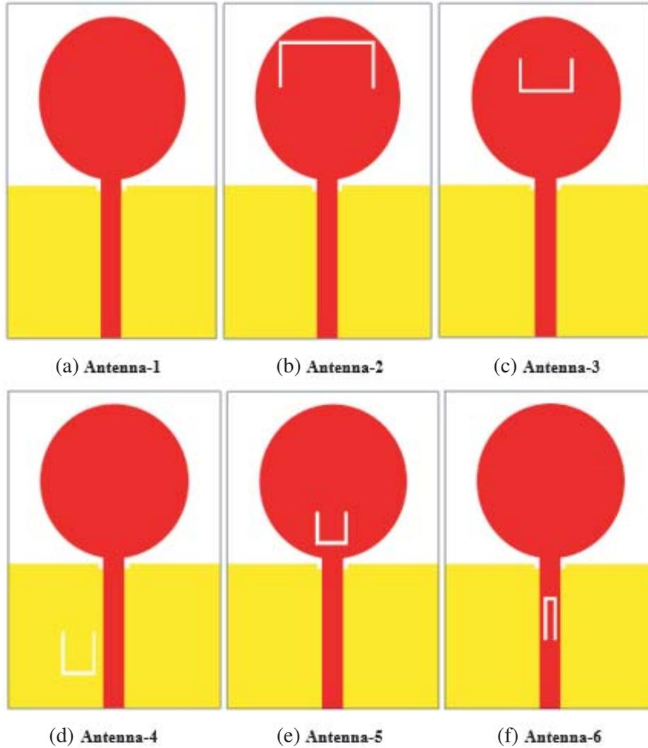
**Figure 2.** Various designs of the proposed UWB antenna: (a) Without notch band. (b) With band notch at ISM. (c) With band notch at Wi-MAX. (d) With band notch at C-band. (e) With band notch at WLAN. (f) With band notch at X-band.
