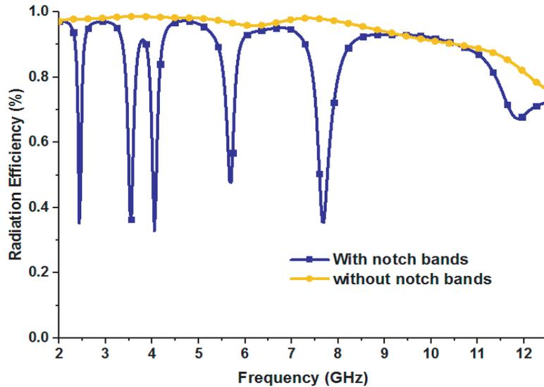
**Figure 13.** Radiation efficiency with and without notch bands.
