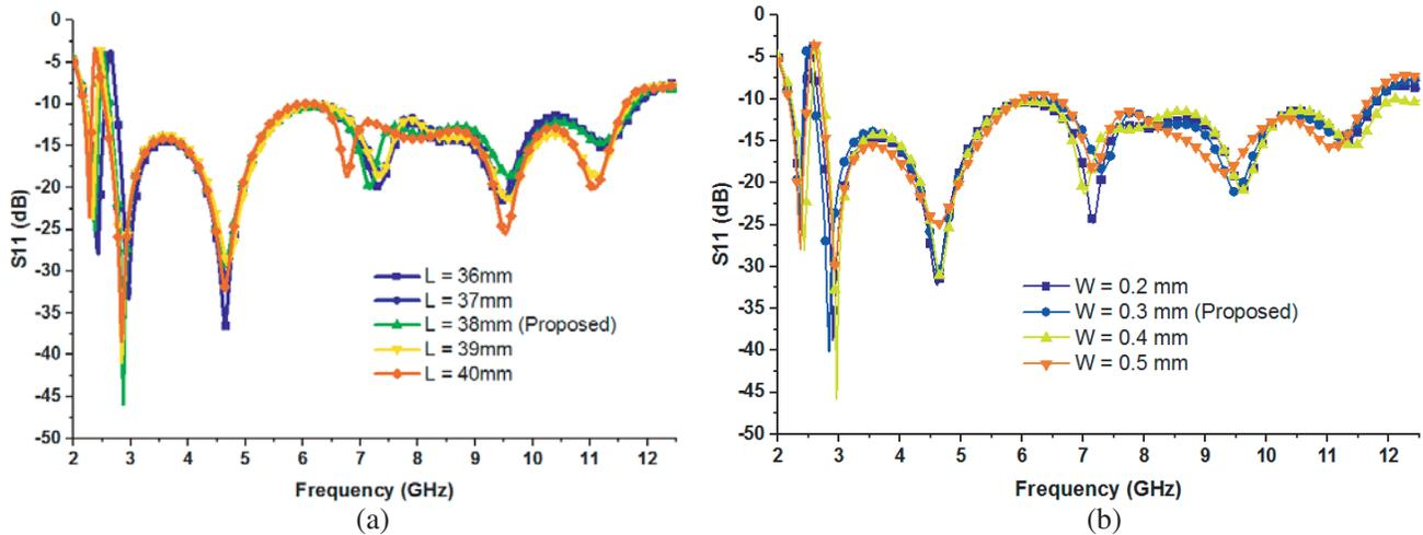
Figure 4. Simulated  $S_{11}$  plot for (a) different lengths of slot-1 (b) different widths of slot-1.
