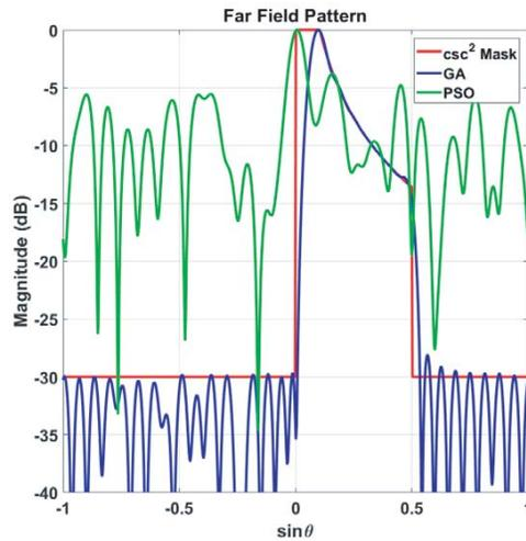
**Figure 6.** Optimized  $\text{csc}^2$  patterns for the  $32 \times 32$ -element array.
