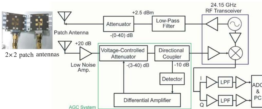
**Figure 2.** Schematic of the 24 GHz reflectometer with an AGC attenuator.
