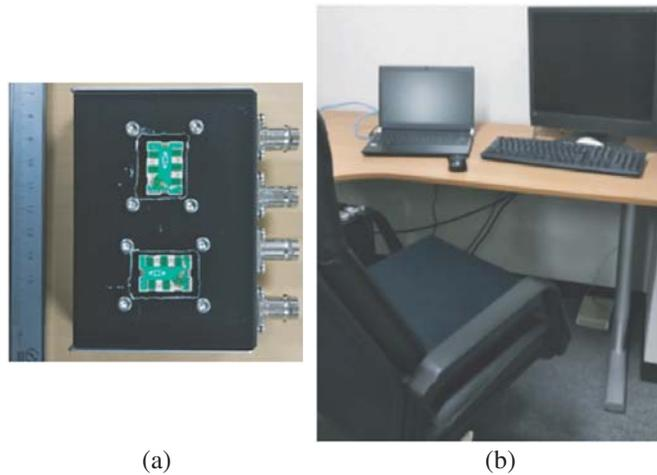
**Figure 1.** (a) 24 GHz radar modules and (b) measurement environment at the office.
