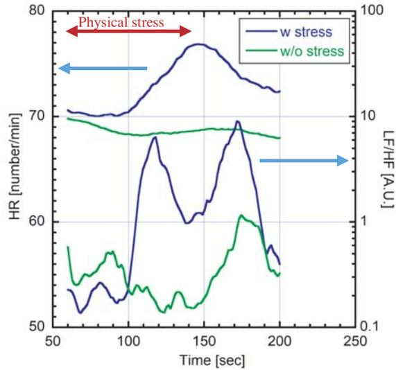
**Figure 3.** Measurement of the HR and LF/HF for two conditions with and without stress.
