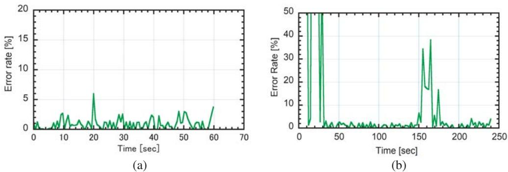
**Figure 6.** Error rate for the condition of (a) idling and (b) high-way driving.
