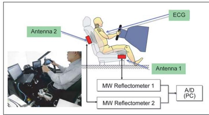
**Figure 4.** Schematic of the experimental setting and picture photo for the test using a driving simulator.
