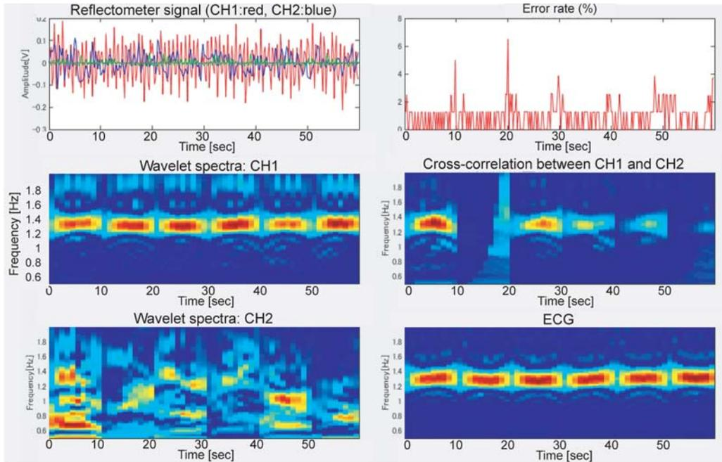
**Figure 5.** Real-time measurement of the HR spectra: (top left) waveforms of reflected signals, (top right) displacement rate of the peak value between microwave ch1 and ECG spectra, (middle and bottom) wavelet transform of microwave and ECG signals.
